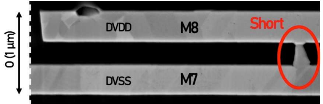
SEM (Scanning Electron Microscopy) cross section of the top two metal layers
