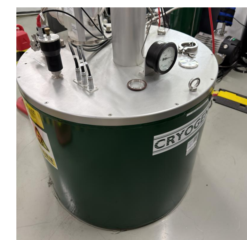
Cryogenic Superconducting Magnet System 2 K, 12 T
