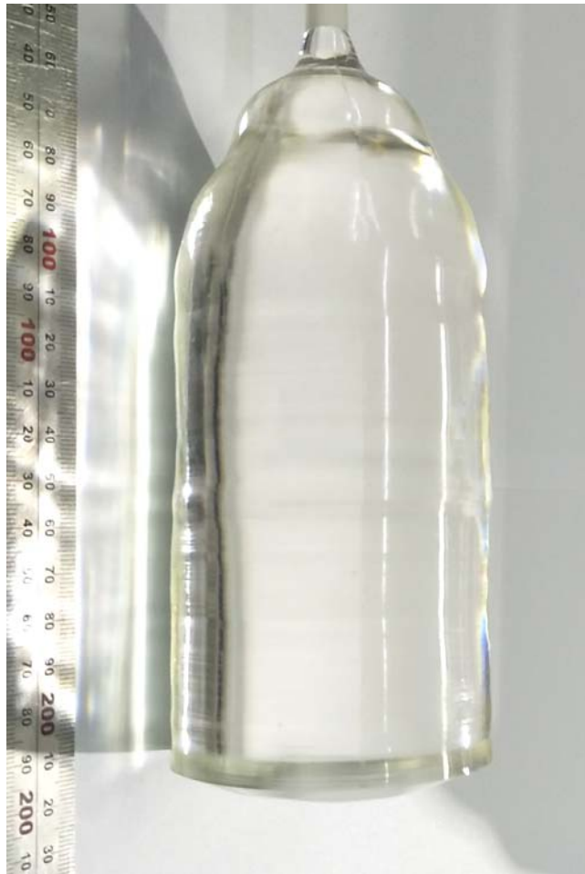
\text{Ø}70\text{-}75 \times 130 \text{ mm}^3 LMO crystal boule (Ningbo University)
