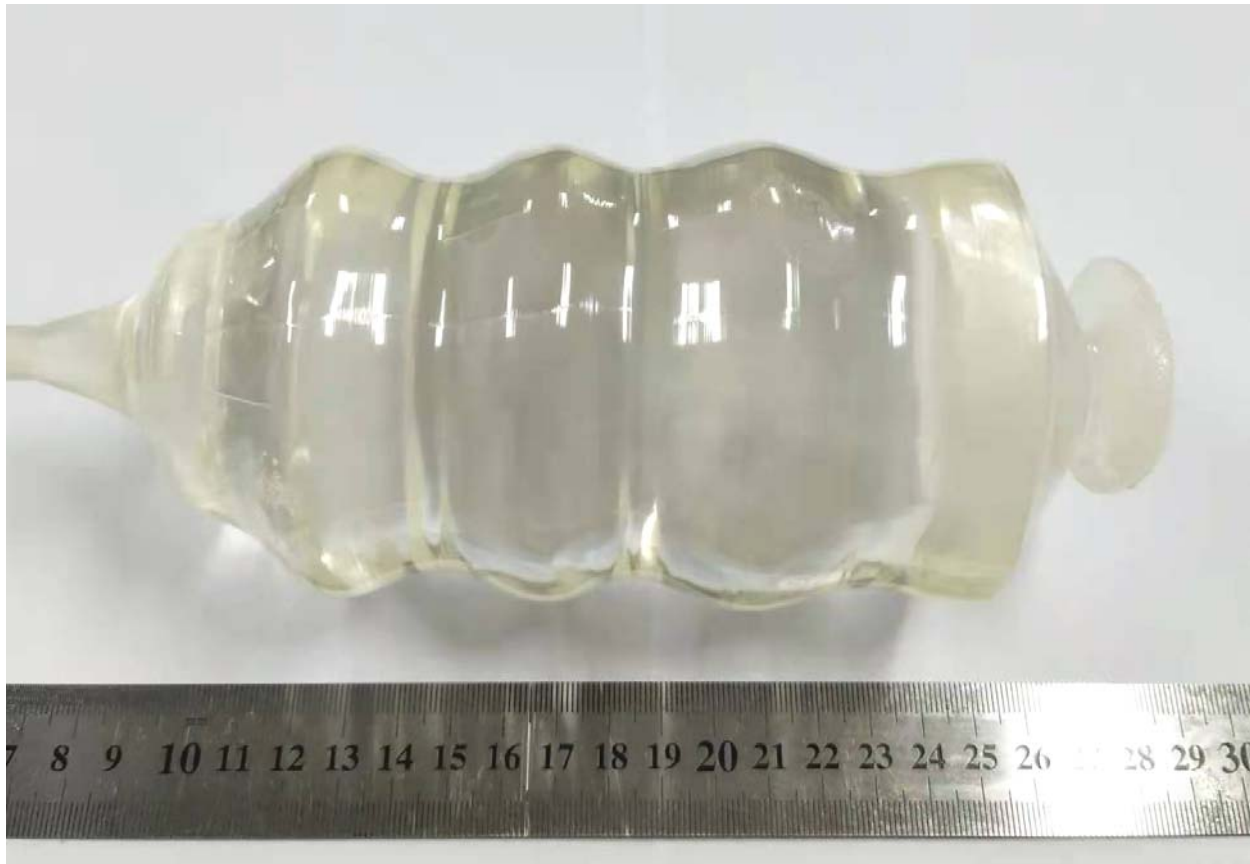
Ø68-75 × 130 mm 3 LMO crystal boule grown in our laboratory (Using refined raw materials)
