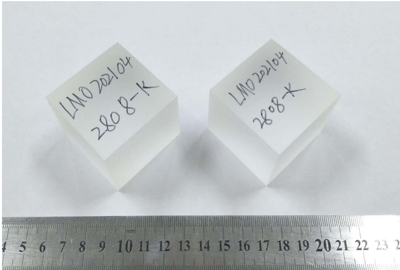
Unpolished LMO cubic crystal elements ( 45 \times 45 \times 45 \text{ mm}^3 )
