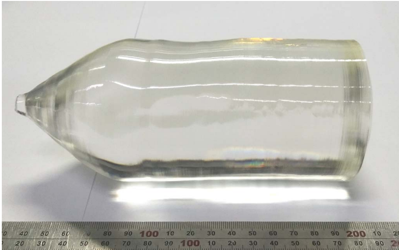
\text{Ø}70\text{-}75 \times 130 \text{ mm}^3 LMO crystal boule grown in our laboratory (Using refined raw materials)
