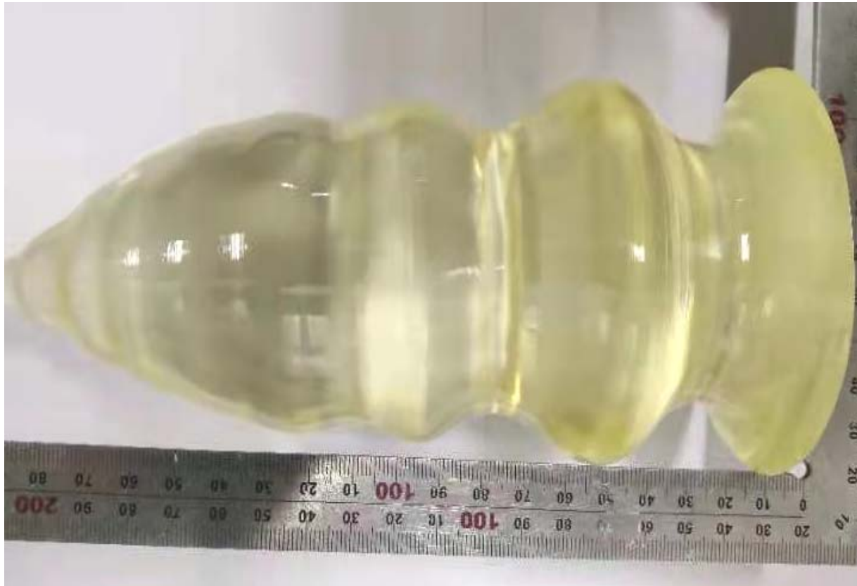
\text{\O}65\text{-}75 \times 130 \text{ mm}^3 LMO crystal boule grown in our laboratory (Using unrefined raw materials)
