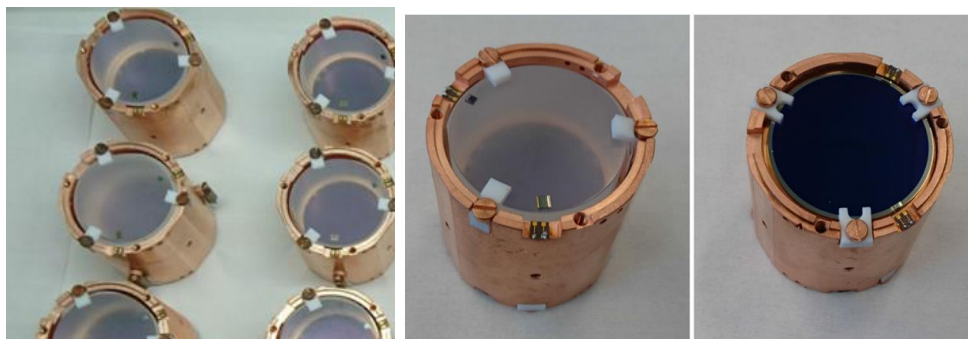
Fig. 4 An assembled CUPID-Mo module. On the left: view from the top, the semi-transparent crystal surface where the NTD and heater are located. On the right: view from the bottom, germanium LD with SiO coating (dark blue internal circle); the 2 mm on the edge of the wafer (17% of the area) are uncoated
